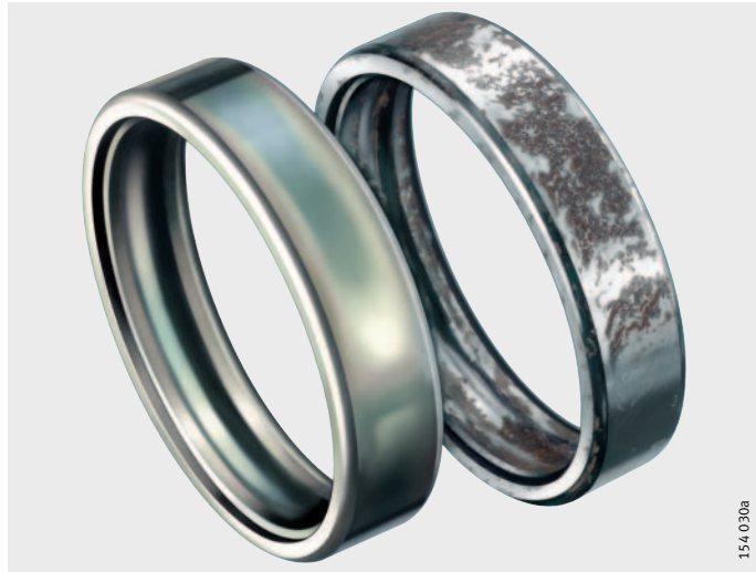
Figure 9 Bearing rings after the salt spray test. Left: a part with Corrotect ® plating; Right: an unplated bearing ring
